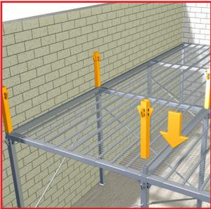
Finally, lift the deck panels one at a time, either around or through the extension and secure into place at the higher level. If required, this process can be repeated across the full structure until the entire platform sits at the new required level. This method negates the need to dismantle and reassemble the platform for use at a greater height.
