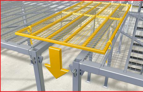
Use make-up panels to bridge gaps of up to 400mm between platforms and secure in place using Rhino Secure Ties, ensuring that the make-up panels are secured at the four corners, one tie at each corner. The make-up panels are designed to be used to bridge gaps between two or more platform systems for non-uniform plots.
