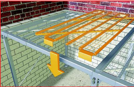
Place Deck Panels on the remaining platforms as shown.
