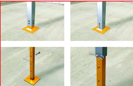
If using the base plate foot extension, select the leg of the right size for the finished platform height, then slide the leg down over the foot to the correct height
